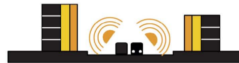
Galleries and facilities provide a "buffer" in the facades shearing the train lines
